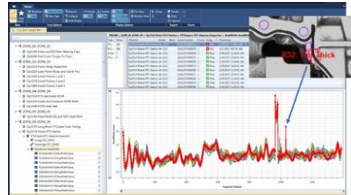
Figure 3. In this image, we present a trend graph of the width of a temperature vulcanizing (RTV) bead that shows a sudden variance in bead width outside of spec.
