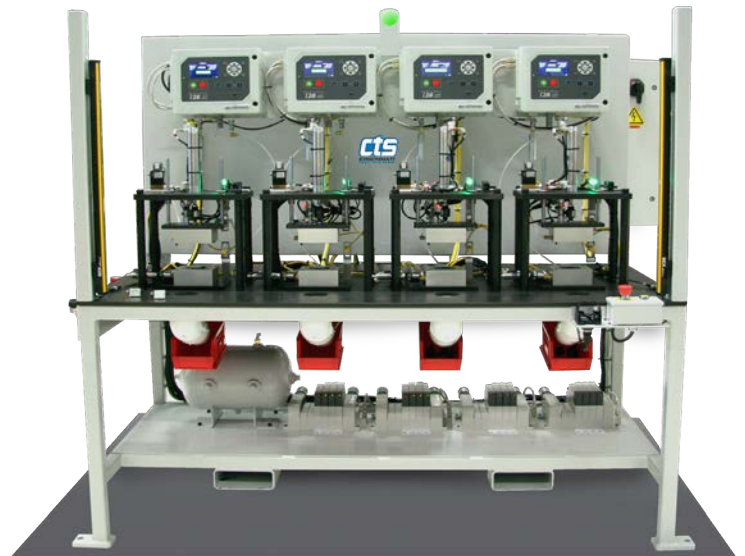
Custom independent CTS 4-station I28 turnkey test system
