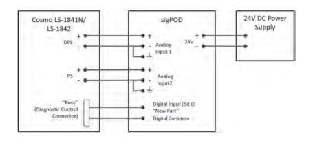
Figure 1: Schematic diagram of electrical connections between sigPOD and Cosmo leak tester.
